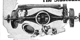
is not merely a "floating" type of axle-but a real FULL-floating rear axle in which the axle housing carries the weight of the
