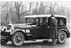
The Safety Chassis of The NEW STUTZ with its worm-gear rear axle brings the body five inches lower than usual; yet full clearance and headroom are maintained.
