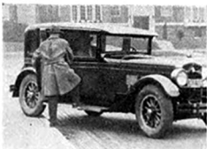
Demonstrating the rigidity of the frame of The NEW STUTZ Safety Chassis. With one wheel on the curb, doors open and close without sticking.
