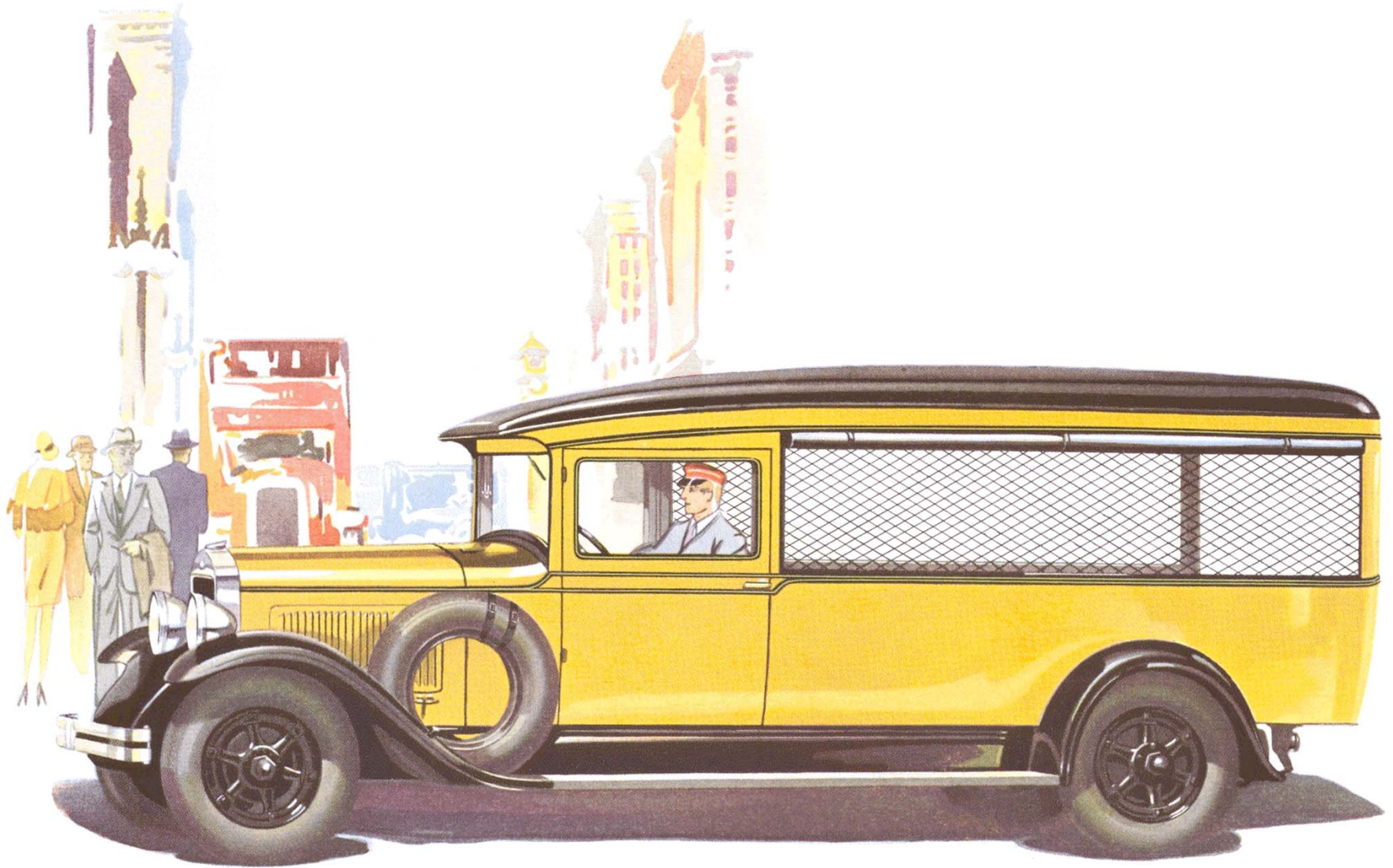
Studebaker Model 40-H Truck, with Screen Body on 4000 Pound Capacity Truck Chassis 146-inch wheelbase »» 68 horsepower engine »» 4-speed transmission 4 optional colors
