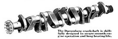
Duesenberg. Two cartridges, each containing 16 oz. of mercury, are attached to the cheeks of the shaft. Since mercury seeks its own level more quickly than any other known element, any periodic vibrations set up in the shaft are counteracted immedi-
