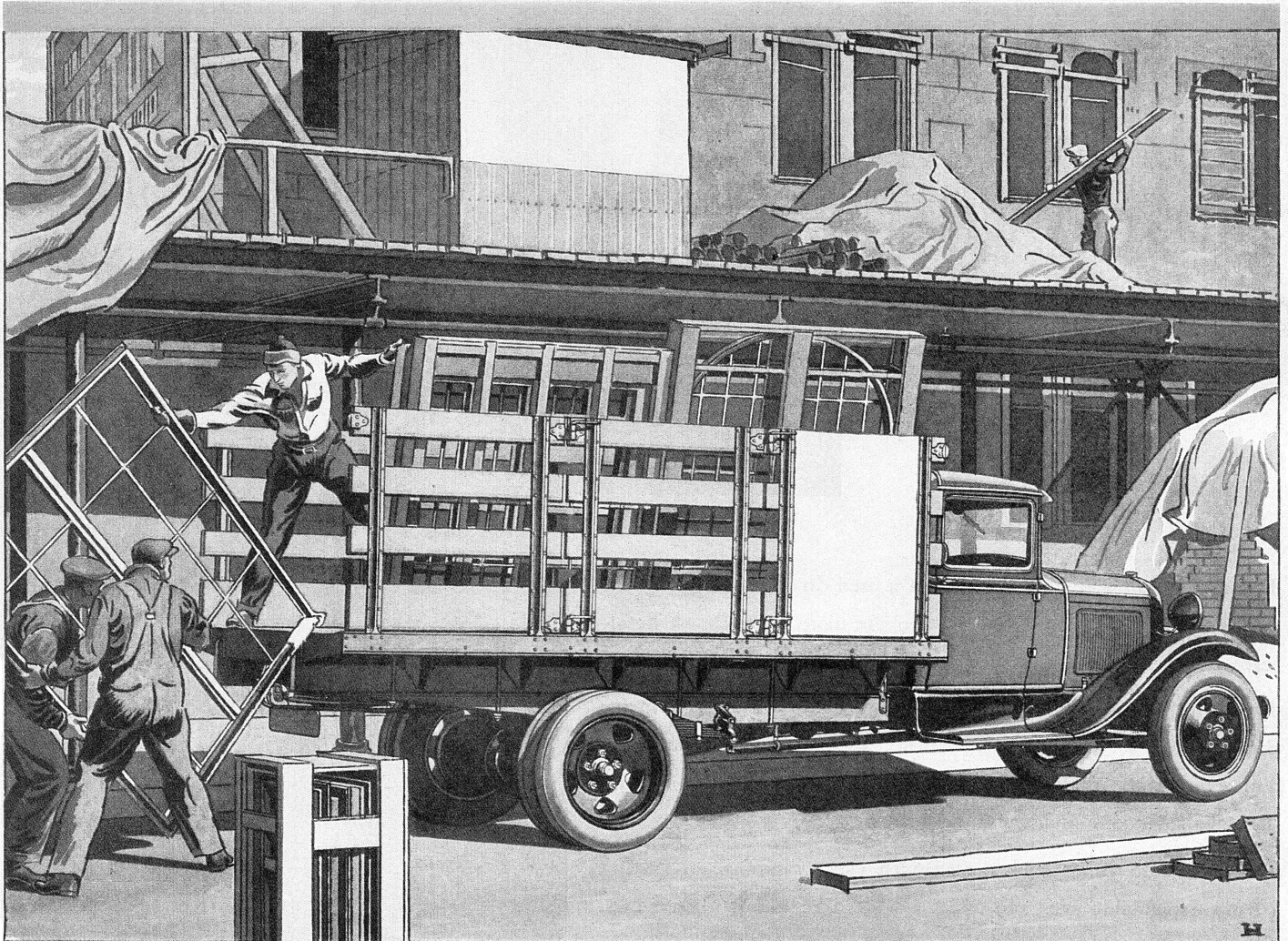
The Stake body on the chassis with 157-inch wheelbase. This type is widely used by manufacturers, contractors and shippers, and for industrial hauling generally.
