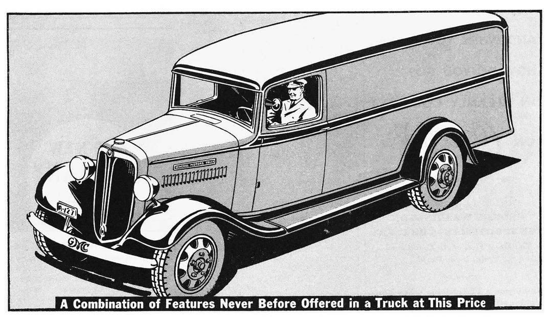
70 h.p. 147 Ft. Lbs. Torque Rifle-Drilled Connecting Rods Electroplated Pistons Removable Steel-Backed Main and Connecting Rod Bearings **Heavy Straight Truck-Type Frame**
