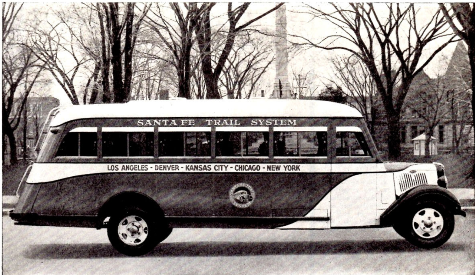
Ford V-8 Bus Unit Equipped with Streamlined Intercity Body
