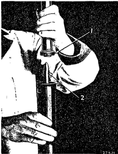
1—Piston rod guide and seal 2—Thimble MT-178
