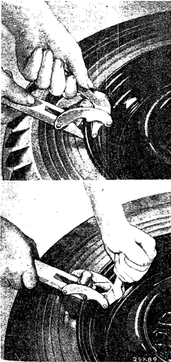
Figure 4—Removing Tire from Wheel with Special Tool C-610—Placing Tool in Position (1941-42 Models)
