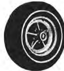
3000 5.803-1373793-WHEEL, CHROME PARTS AVAILABLE SEPARATELY 5.871-1376689-MEDALLION AND BEZEL (TRI-SHIELD)
