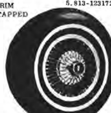
LE SABRE & CENTURION WIRE WHEEL COVER 5.858-981696-COVER 5.871 - 1241629 SPOKE (LONG) 5.871 - 1241631 SPOKE (SHORT)
