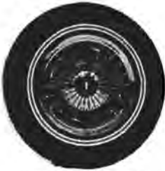
30-4000 WIRE WHEEL 5.858 - 981270 - COVER 5.871 - 393240 - SPOKE (INNER) 5.871 - 393241 - SPOKE (OUTER)
