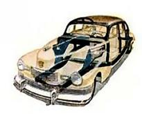
Product of Nash research and engineering, new Unitized ' body-frame construction sets the pattern for construction, Built a new way, with frame and body welful into a single steel-girdered unit, it is lighter and immeasurably stronger. 8500 spec welds eliminate noise-making joints.
