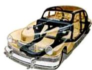
Product of Nish research and engineering, new Unitized body-frame construction sets the pattern for tomorrow. Built a new way, with frame and, body welfed into a single steel-girdered unit, it is lighter and immeasurably stronger. 8500 spot welds eliminate noise-making joints.
