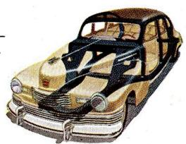
Product of Nash research and engineering, new Unitized body-frame construction sets the pattern for tomorrow. Built a new way, with frame and body welded into a single steel-girdered unit, it is lighter and immeasurably stronger. 8500 spot welds eliminate noise-making joints.
