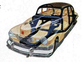
Product of Nash research and engineering, new Unitized body-frame construction sets the pattern for tomorrow. Built a new way, with frame and body welded into a single steel-girdered unit, it is lighter and immeasurably stronger. 8500 spot welds eliminate noise-making joints.
