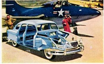
Here's the basic secret of streamliner trains, modern airliners and Nash automobiles. Airflyte Construction welds body-and-frame into one double-rigid, girdered unit that's safer.
