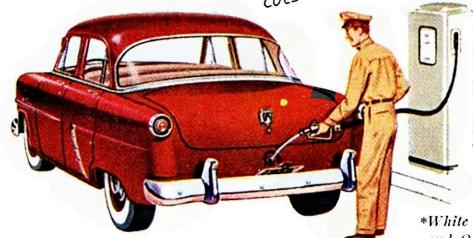
New Centre-Fill Fueling makes "filling-up" convenient from either side of the pump. And with no long filler pipe in the way, the luggage compartment is a suitcase bigger. The rear license plate is hinged to conceal the gas cap.
