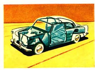
Like Airliners, the Aero Willys is built with body and frame made as one unit, welded together—extra strong, safe and rigid.
