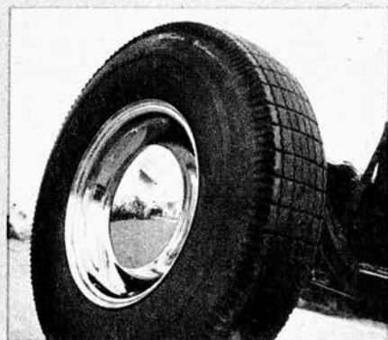
Chrome plated rear wheel is wide base Lincoln rim reversed on Merc center.
