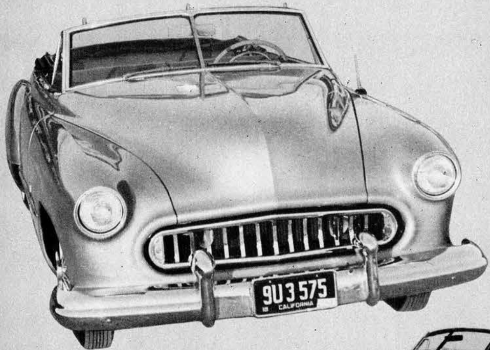
Alterations of front includes frenched headlights, hand made grille and protruding oval shell, and Merc bumper.
