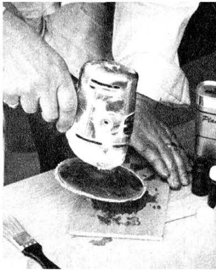
Step 7. Within 15 minutes after last step the resin is set up hard enough to smooth out. Bill is using a disc sander because of hardness of resin.
