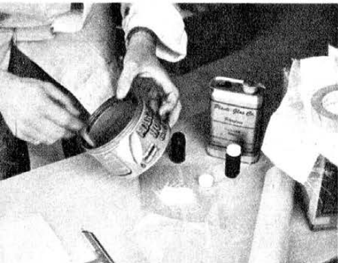
Step 4. Resin and Catalyst are being thoroughly mixed in clean coffee can
