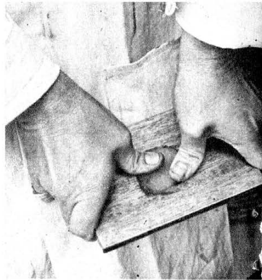
Bill demonstrates how fiberglass and resin has adhered to plywood only 30 minutes after start of demonstration
