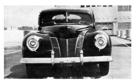
PROFILE is low and neat with chopped top, channeled body and normal fender line
