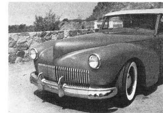
GRILLE was made from short lengths of chromed tubing welded into place
