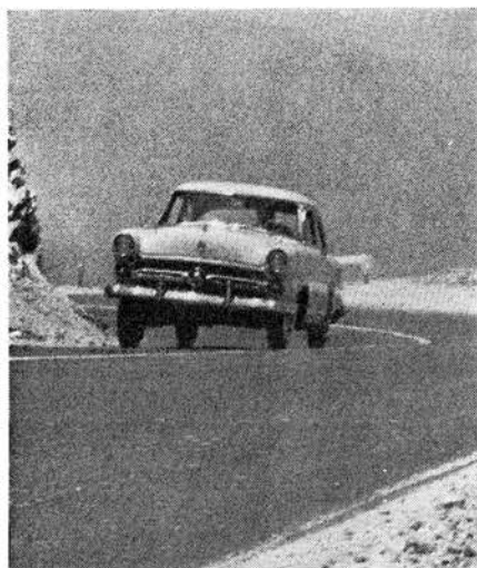
SUSPENSION weakness was noted immediately. Extra weight of Cad engine necessitates installation of stiffer springs
