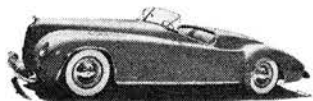
Cadillac powered MAVERICK SPORTS Plush 123" wheelbase car with 16'6" Fiberglas body constructed by Industrial Plastics Service, Oakland, Calif.
