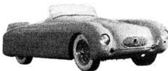
Le Blanc-Bardahl Streamliner. Fastest car in America. 24'6" Fiberglas streamliner, designed by Gene Le Blanc. Body constructed by Industrial Plastics Service, Oakland, Calif.
