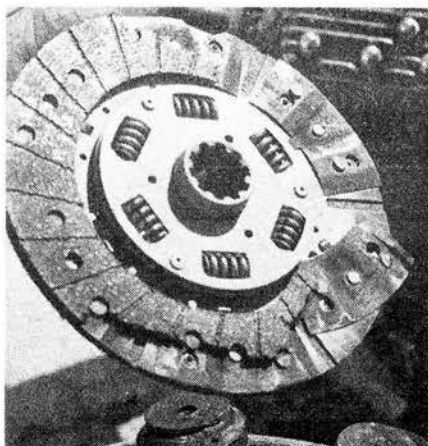
CLUTCH disc taken from the Meredith-Barton B coupe after four hard days
