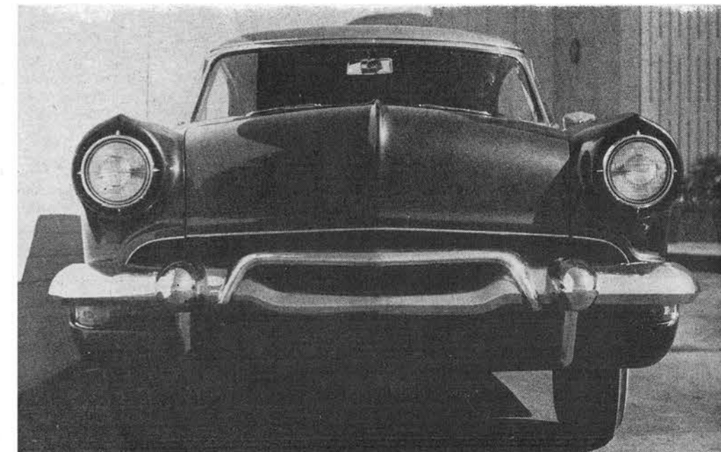
Panel under bumper, formerly chrome, was moved back three inches, then painted
