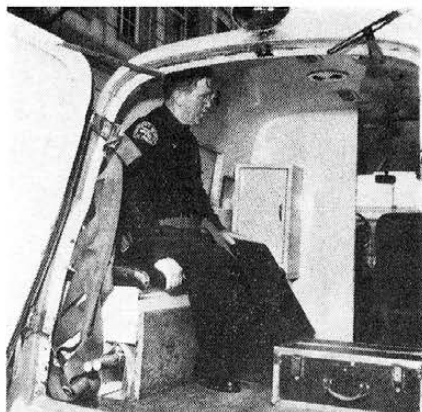
Rear seat belt as installed in Los Angeles' City Ambulances is demonstrated by Chief Attendant Howard Roberts. Gilson belt attached to door frame at left
