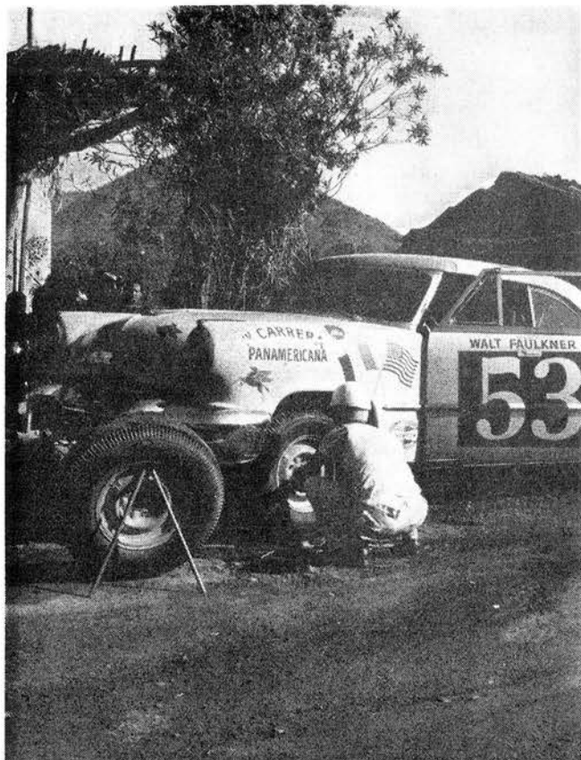
Study in scientific preparation: Lincoln tire stop en route. Note waiting tire propped on simple bipod. "LF" painted on rim implies infinite attention to every detail to save time
