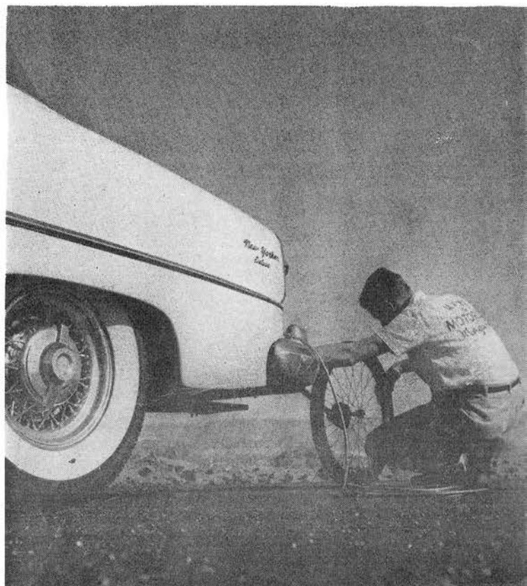
Test crew member makes adjustment of fifth wheel prior to speedometer calibrations and acceleration runs. Speedometer was exceptionally accurate at most speeds, errors being slight
