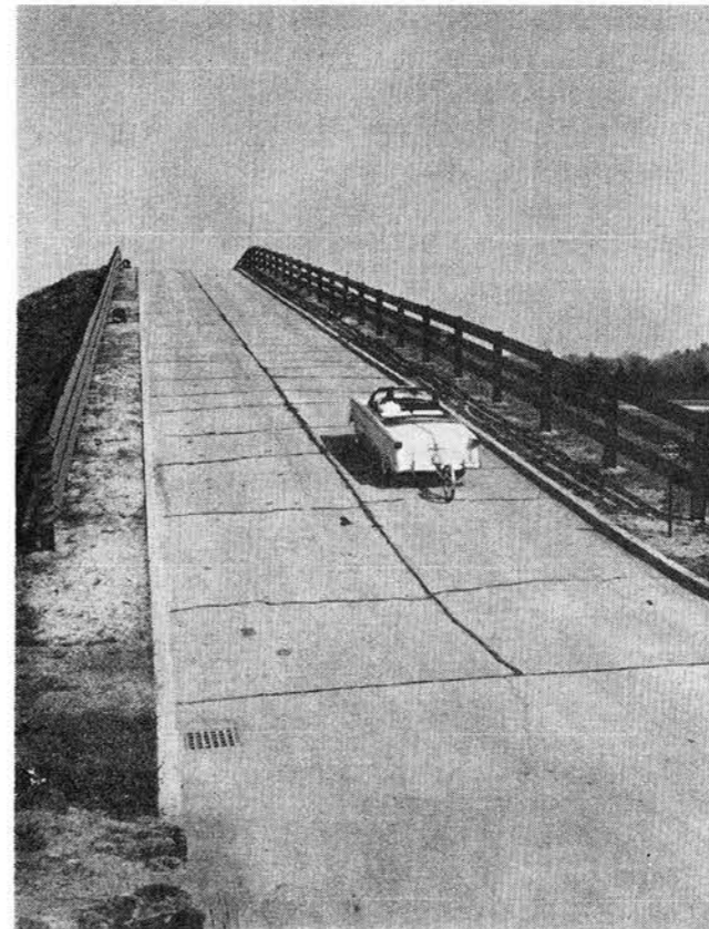
Trailing a fifth wheel, a Ford convertible samples the pulling power of the new ohv V-8 on the 17 per cent grade of an artificial hill at company's proving ground track
