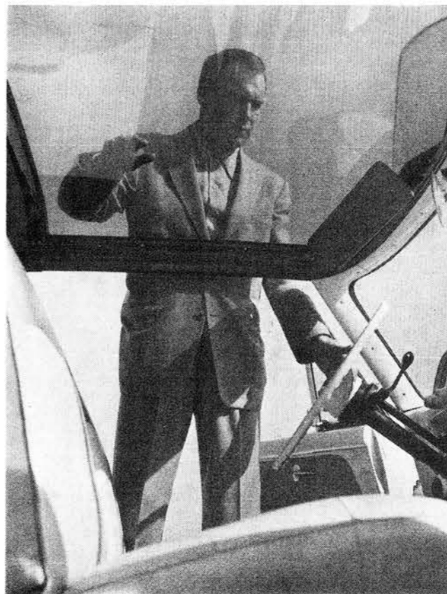
Test driver has a look at the new plexiglass top which is tinted to eliminate most of heat rays from the sun. Overall view of the model showing styling is at top of opposite page
