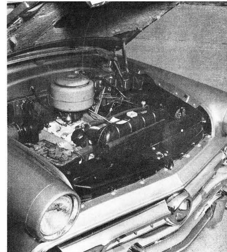
Switch in engines has had good and bad points from accessibility angle. However, the change in the suspension and frame clears oil pan area, permitting much easier removal
