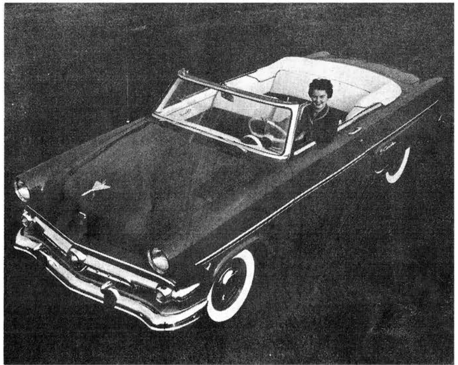
Overall view of '54 Crestline convertible shows that Ford has retained the basic styling lines that proved so popular in 1953. The long, clean look is unchanged and minor refinements made in grille and trim are designed to give the car a lower and wider look. Note the new transparent plastic speedometer in front of the steering wheel
