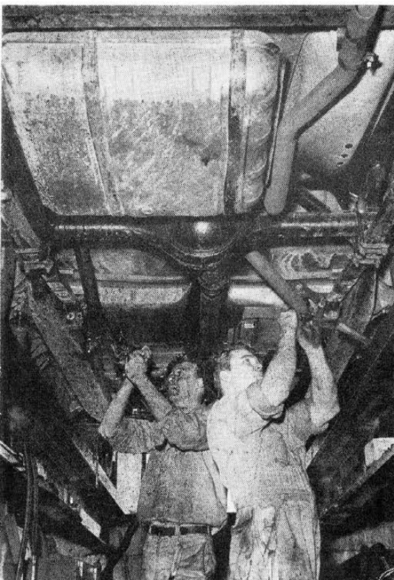
After initial test and preliminary to the final one, stock exhaust (right) was replaced with improved system (left)
