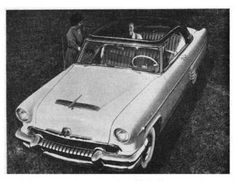
The '54 Mercury Monterey "Sun Valley" may start a new styling trend with its plexiglas top in forward roof area. Made of quarter-inch material tinted green to minimize light glare, it is the first American production car of its type
