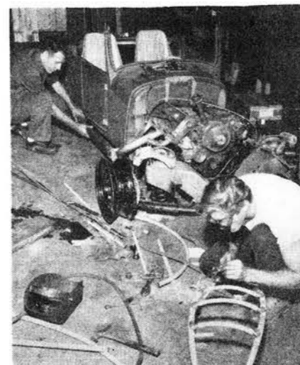
Amid litter of final preparations, Ak Miller (left) installs outside headers, while Pinky Farina makes grille from strong three-quarter inch steel tubing
