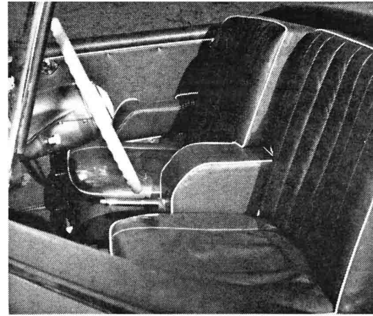
Thickly padded seats and curved backrests are a boon to long distance motoring. Center armrest can be removed for added space
