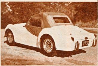
the late and unappreciated Crosley Hotshot. The car is solid, its steering is quick, its four-speed floor shift is right there when you want it, and it has good manners in the corners. Its more-than-adequate 90 bhp comes from a four-cylinder, two-carburetor ohv engine that just stays inside the two-liter class with its 121.45 cubic inches. Overdrive is optional.
