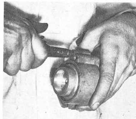
• Front band servo is checked by air pressure at apply hole. Piston should snap smartly into engage position. Upon release, it should return sharply.
