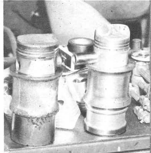
● New pistons were cast to Ernie's own design with high crowns giving 8.2/1 compression.
