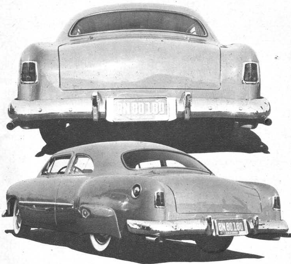
● Adapting '51 Chrysler rear fenders added 6-ins. more overall width. Rear bumper is from front of '53 Ford which has section removed from the center and replaced with flat plate, making neat license mounting and also was needed for extra width. '53 Ford Ranch Wagon bumper guards are installed and taillights are '51 Chrysler. Body seams have been filled-in and deck lid shaved.
