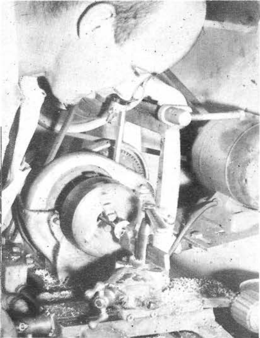
● Entire valve train was lightened in process of souping. Here Ernie tulips a valve on lathe.
