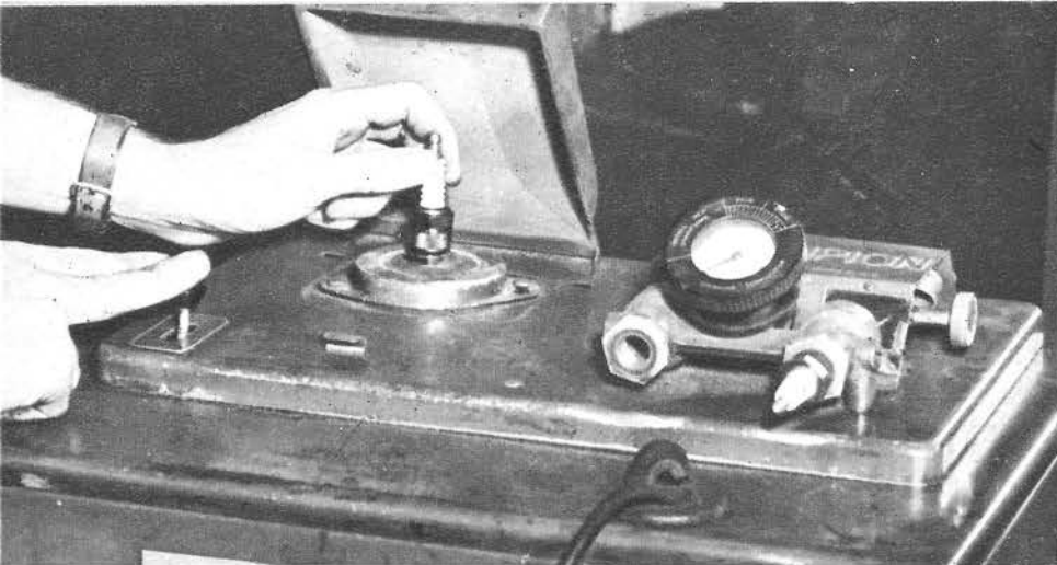
• Carbon deposits are easily removed by sand blasting in cleaner. Sand must be blown out with air.
