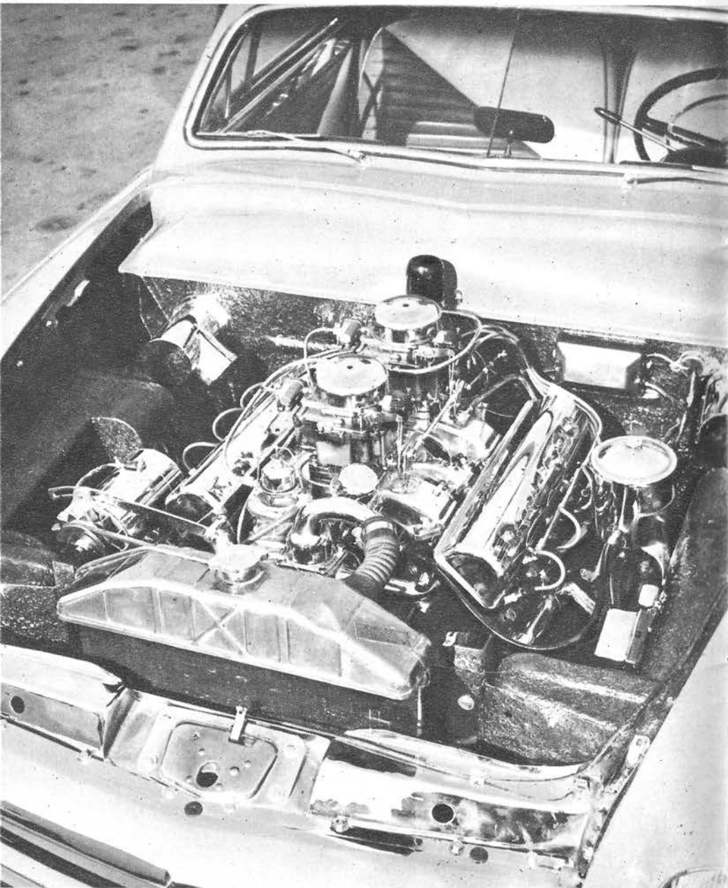
● Exterior of the semi-race Cad is equally as beautiful as the restyled body. The firewall and inner fender panels are sprayed with dum-dum and painted a dark blue, making an elaborate contrast against the chrome goodies on the mill and the orange body paint. The hood is being rebuilt to clear the carburetors and is not completed as yet. Note windshield was butt-jointed and sealed with plastic.
