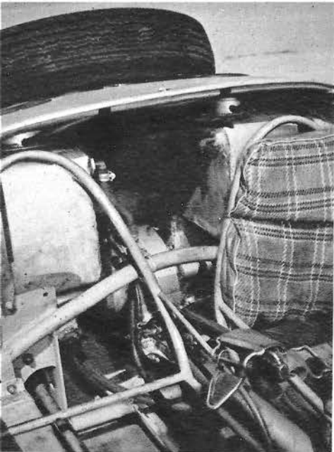
● Seats are tube skeletons. Rear end is Pat Warren riding between MG TD axle housings. ● Dry sump oil tank is placed beneath passenger seat. Note small, light frame tubing.
