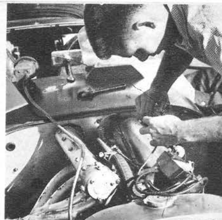
● Pit crewman adjusts ticklish Amal motorcycle carb, soon to be exchanged for Carter.
