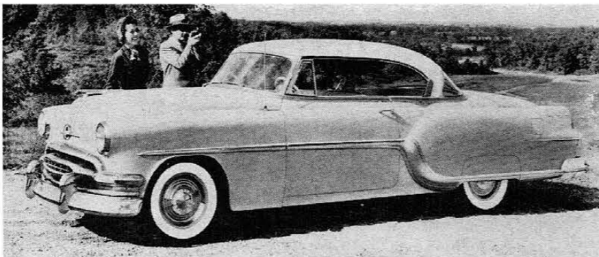
Pontiac has new series in Star Chief. Catalina model shown here is a big car, mounted on a 124-inch wheelbase, and is powered by familiar inline eight engine
