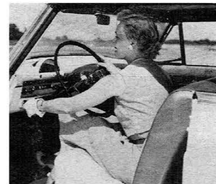
Plastic speedometer raised on recessed dash is novel and improved feature on Fords. Burnished metal is non-reflecting
