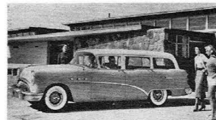
All-metal estate wagon is new to the Buick line for '54 and is shown here in Century series. Engine is the 200-hp Roadmaster V-8, wheelbase is 122 inches
