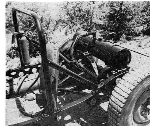
Roll bar bolted to the frame is braced to rear. Rear cross member and shock mounts are 3-inch tubing, \frac{1}{8} -inch plate
