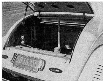
Inset taillights are from '49 Ford. A '47 Stude convert top motor lifts deck
