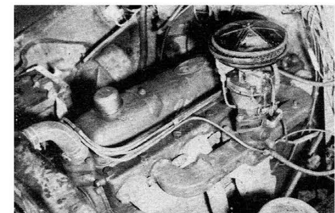
To keep his Chevy in line with his dad's higher horse-powered Cadillac, Tommy installed a GMC 270 for greater power. Conversion is a good one as change-over entailed no compartment changes for good power-to-weight ratio
