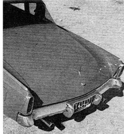
Modifications to the rear are limited to rounding the deck lid corners, removal of unnecessary trim and seam frenching
