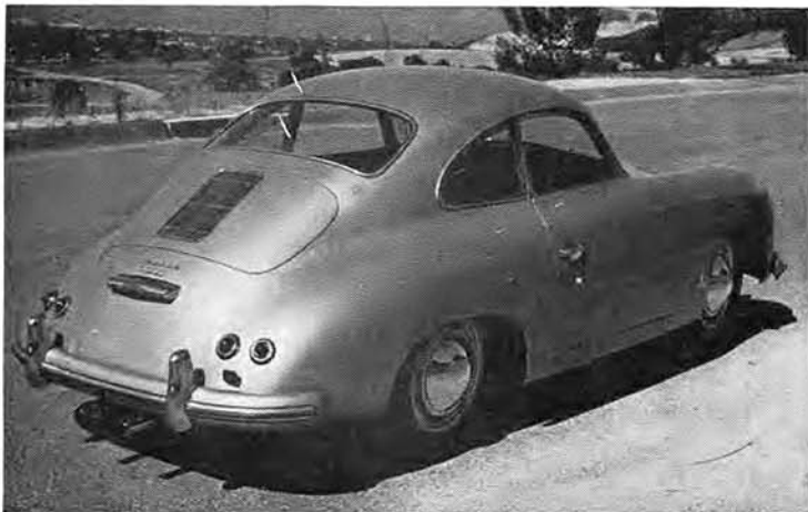
Air-intake on the rear deck is the only clue to engine location.
