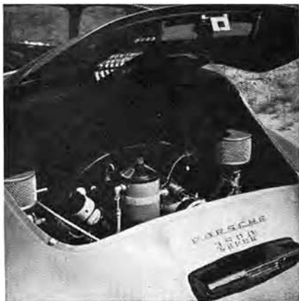
Rear mounted engine is accessible for tune-ups, yet can be "dropped" in 20 minutes.
