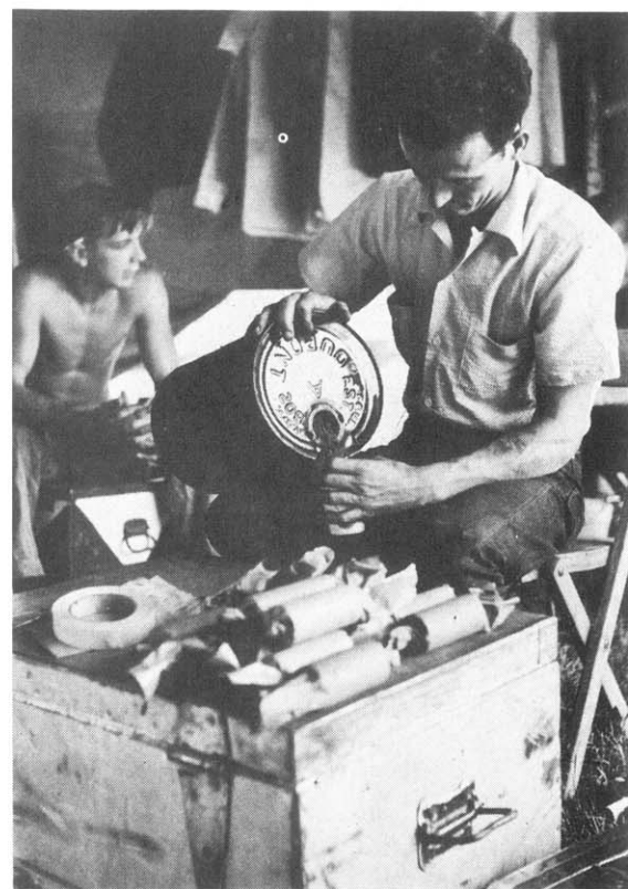
Pouring black powder into JATO cases is Wally Hall's job before the Hell Drivers really "shoot the works."
