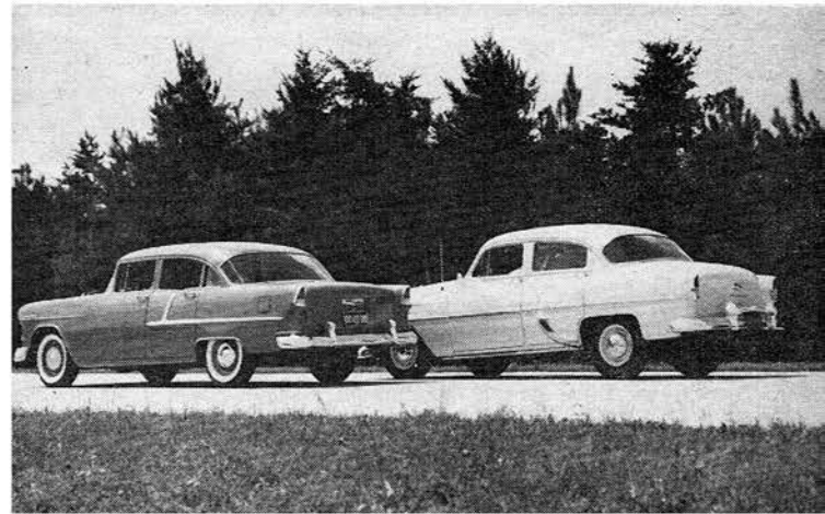
1955 models have ball-joint front suspension with "anti-dive" features. Note how '55 model stays level, '54 "dives" braking.
