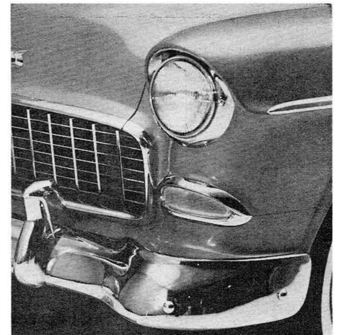
Frontal treatment of the 1955 Chevrolet features inward slope, Ferrari-type grille, hooded headlights and wrap-around bumper.
