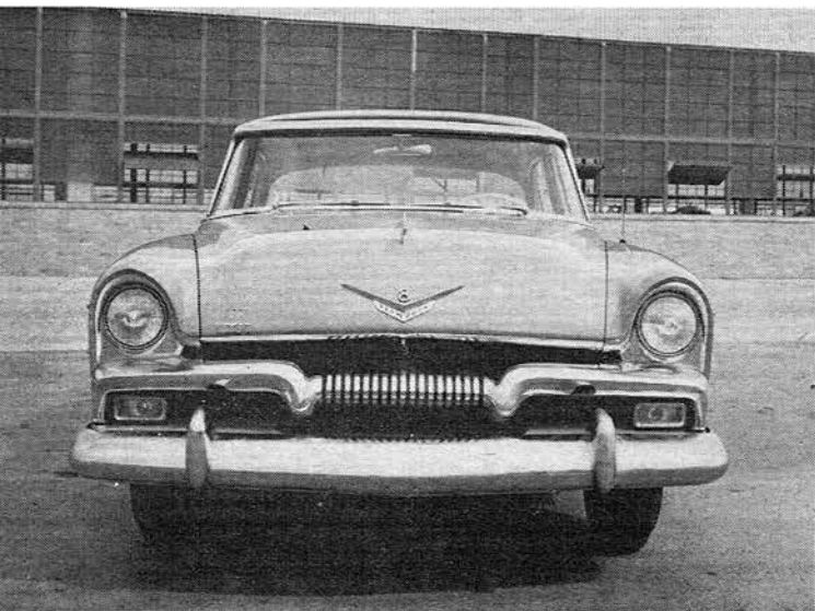
Body styling is based on look called "tumble home" design. Slant of top section helps concentrate weight in lower areas.
