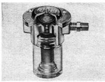
FILT-O-REG is the only available fuel filter and fuel pressure regulator, the manufacturer claims. It supplies filtered fuel to your carburetor at a constant 2 pounds pressure and eliminates flooding and fuel waste. It is made for use with gasoline, alcohol, kerosene and other fuels. Bell Auto Parts, 3633 Gage Avenue, Bell 7D, Calif. Std. Model \$7.95.
