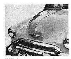
NOW there's an easy way to shave your hood. It's done with a full length Bull Nose molding, which California Custom Accessories Mfg. Co. claims is the only full length molding in America. It is of polished stainless steel and can be painted if desired. No holes to drill, no cutting. From manufacturer, 301 W. Jefferson Blvd., Los Angeles, California.
