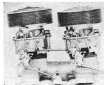
THE NEW Nicson dual-quad manifold is available to fit '49 through '54 models of Cadillac and Oldsmobile. Equipped with linkage designed for Hydra-Matic, they provide up to 25% more hp which means more acceleration and speed. Prices and details sent upon request from Nicson Engineering, 4552 E. Washington Blvd., Los Angeles, California.
