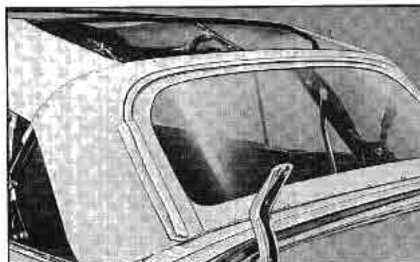
Fig. 3-110 Tacking Back Curtain to Rear Bow
