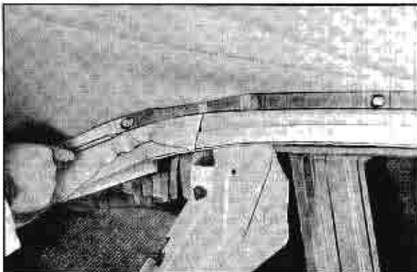
Fig. 3-113 Marking Position of Back Curtain and Top
