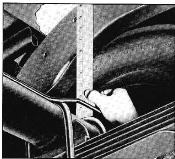
Fig. 6-5 Measuring Rear Spring Height
