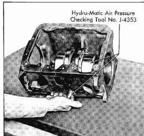
Fig. 14-4 Checking Clutch Hydraulics
