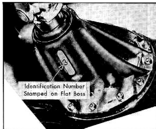
Fig. 1-5 Rear Axle Gear Ratio Identification Number
