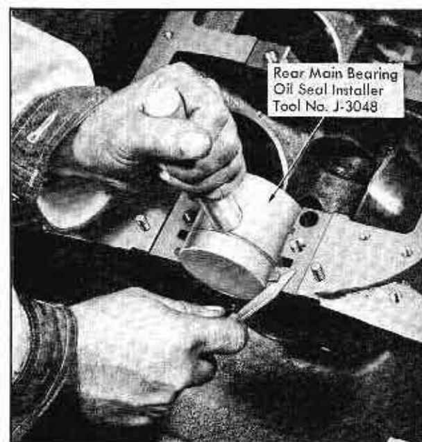
Fig. 10-29 Cutting Rear Main Bearing Oil Seal
