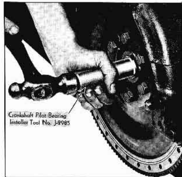
Fig. 10-34 Installing Crankshaft Pilot Bearing
