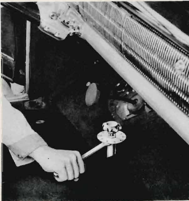
Fig. 4. Adjusting bands external method
