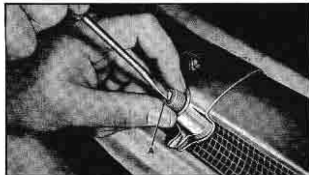
Fig. 3-4 Windshield Wiper Cable Tension Adjustment
