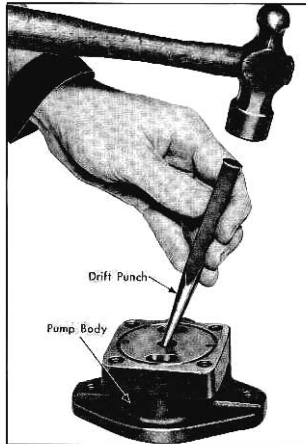
Fig. 7-20 Removing Shaft Bearing
