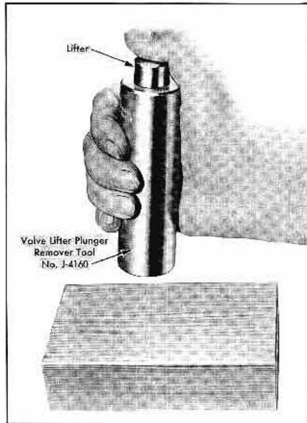
Fig. 10-14 Removing Stuck Plungers From Body
