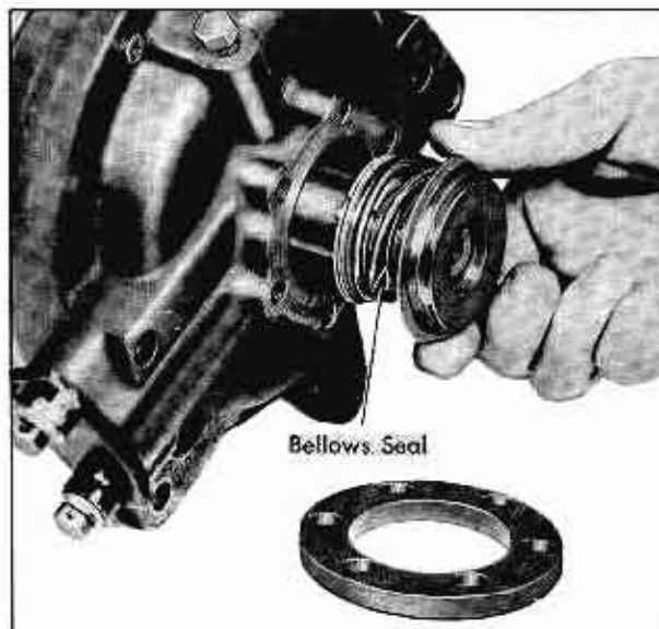
Fig. 16A-24 Removing Bellows Seal
