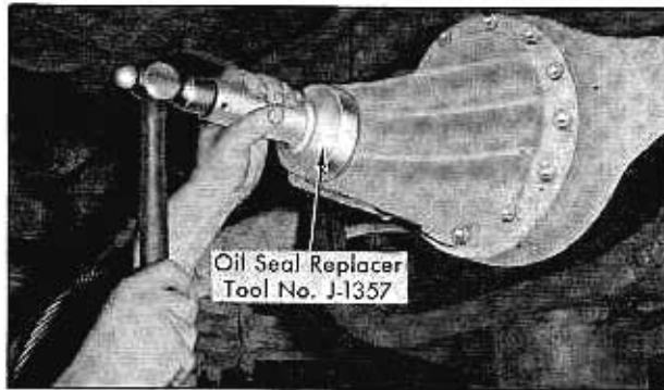
Fig. 8-6 Installing Pinion Oil Seal
