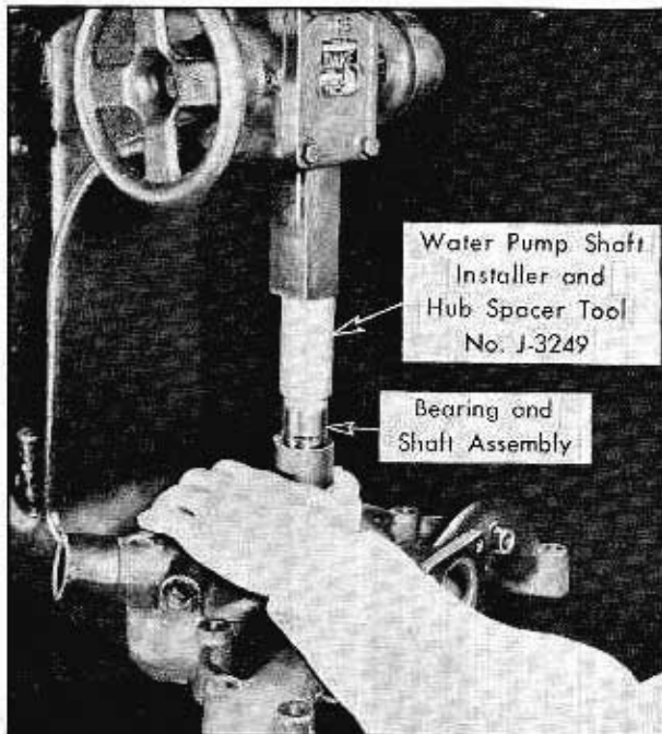
Fig. 13-7 Pressing Bearing and Shaft Into Pump Housing
