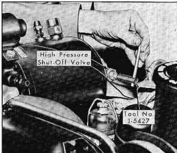
Fig. 16A-12 Closing High Pressure Valve
