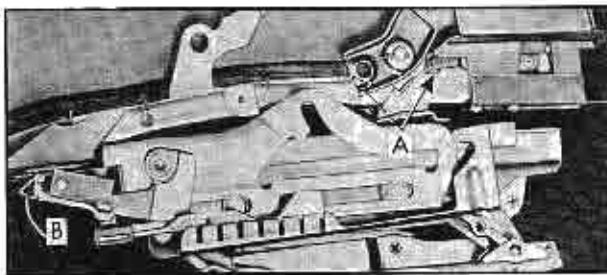
Fig. 3-60 Detaching Seat Assembly from Adjusters (Coupes)
