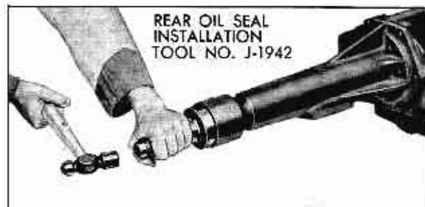
Fig. 14-47 Installing Extension Housing Oil Seal
