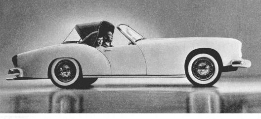
When not in use, the entire top folds neatly into the rear deck, completely out of sight, providing the dramatically clean lines that distinguish the new KAISER-DARRIN Model KF-161.
