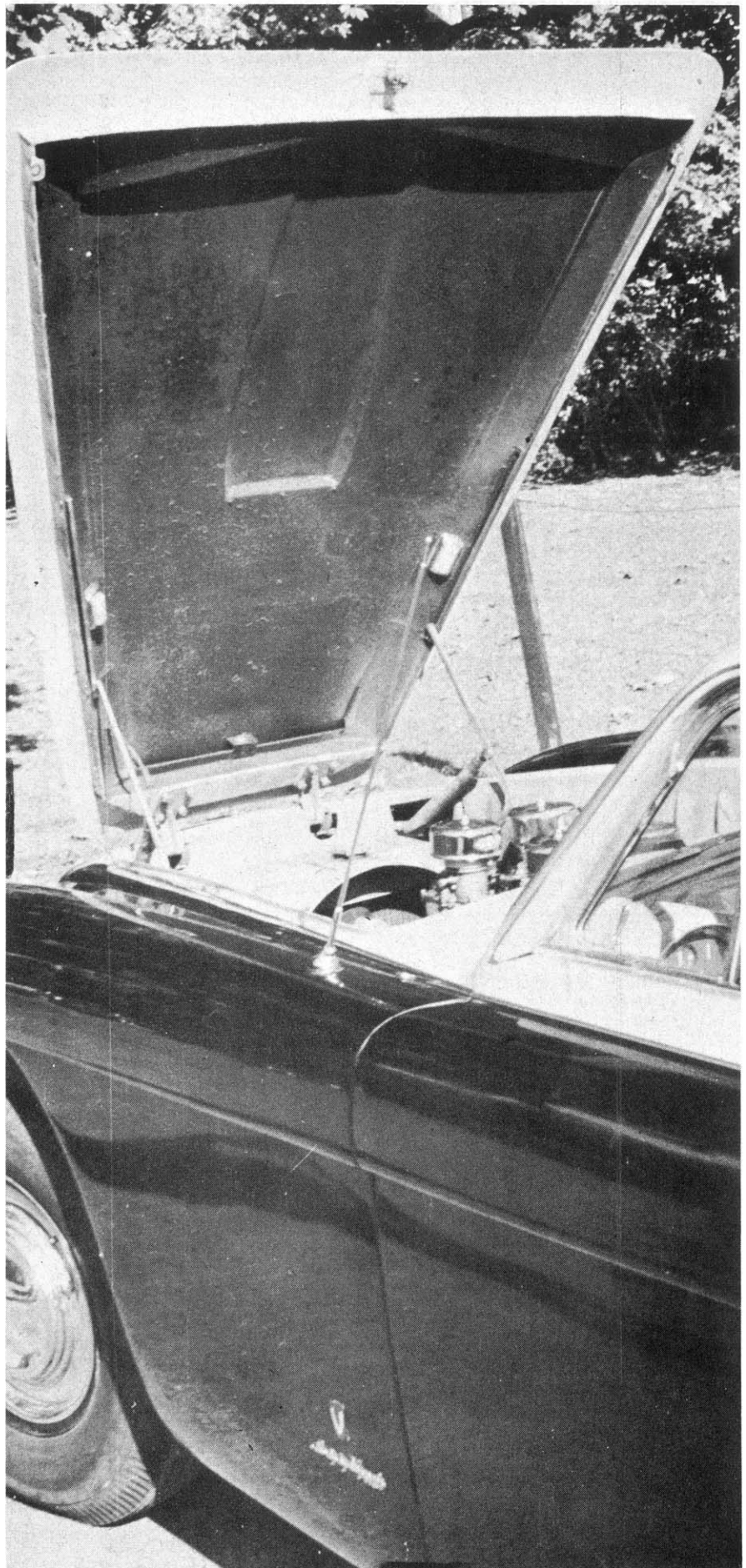
Front-hinged hood provides easy access to engine.
