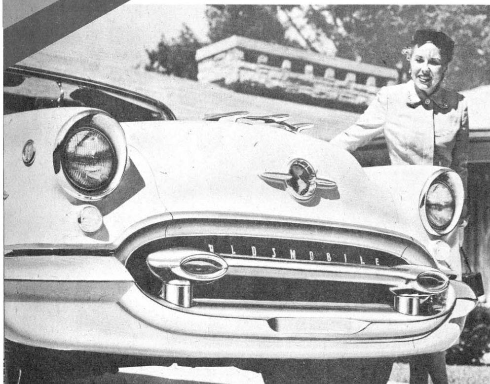
Entirely new front end styling marks the 1955 Oldsmobile. Contour of the front bumper has been redesigned to harmonize with the styling, headlights have been recessed and parking lights are bullet-shaped. Hood sports a new world emblem.
