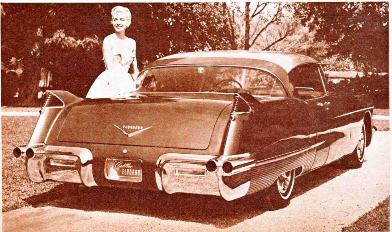
Projectile-shaped rear fenders flow back into outer rear bumpers forming the "quad" exhaust system. Note back-up lights
